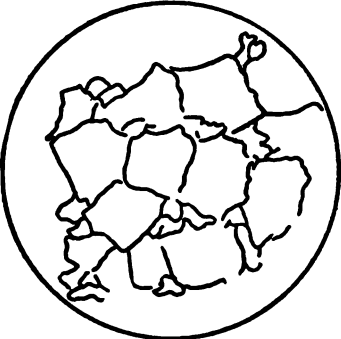
INTERPRETATION OF GRAIN STRUCTURE IN SCHOEN WHEEL AT VARYING DISTANCES BELOW SURFACE OF TREAD.
